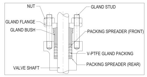
This Gland Packing consists of 1 Rear Packing Spreader, 1 set of V-PTFE Gland Packing and 1 Front Packing Spreader.
