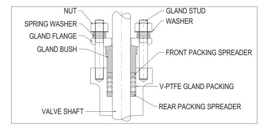
This Gland Packing consists of 1 Rear Packing Spreader, 1 set of V-PTFE Low Fugitive Emission Packing and 1 Front Packing Spreader.
